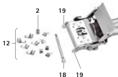
Fig. 1 Flap rod dismantled
