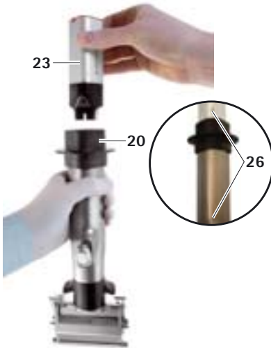
Fig. 4 Installing the sterile funnel in the battery compartment
